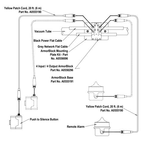
3. Attach one connector of a yellow patch cord to the terminal on the alarm silence switch module. Tighten the cord grip ring until snug.
